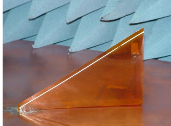
Figure 1 Vee monopole with discrete 249 \Omega resistor.
