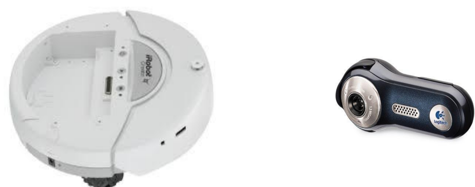
The iRobot Create and the Logitech Quickcam Fusion are the simplistic and low cost components used for this VO system.
