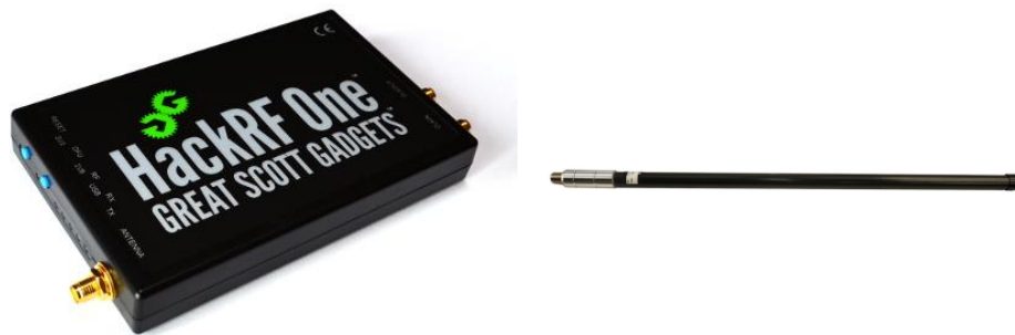
Fig. 3, The HackRF One [10] and 1090 MHz antenna [1]
