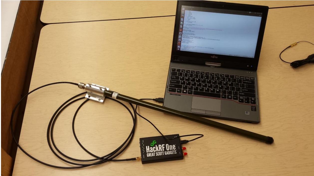
Fig. 6 – A HackRF One equipped with a 1090 MHz antenna, connected to a laptop running the ADS-B program.
