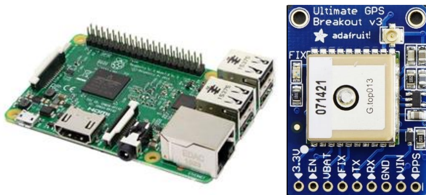
Fig. 4, Raspberry Pi 3 Model B [15] and GPS module [2]
