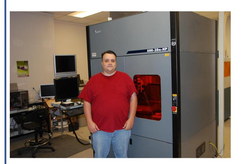
nScrypt machine in the direct print lab at South Dakota School of Mines & Technology. This machine will deposit the ink following our antenna profiles.
