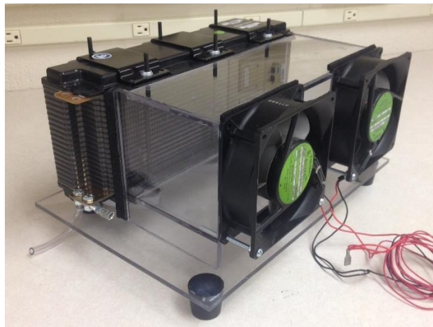
Figure 6. The stack enclosure/mounting fixture with the stack and fans mounted [3]
