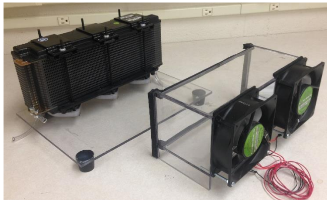
Figure 7. The enclosure/mounting fixture has two unconnected parts [3]
