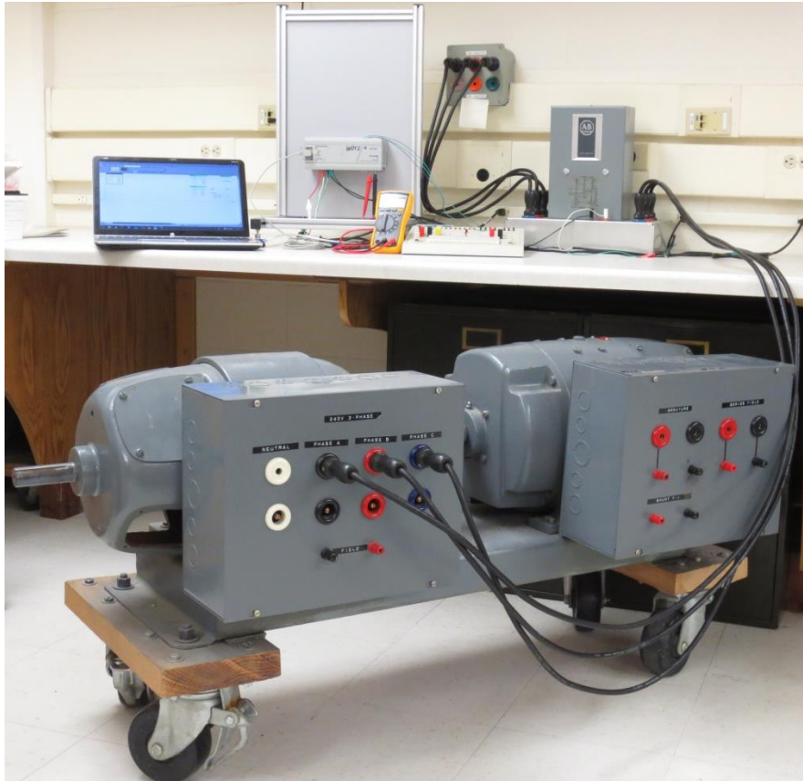
Image of setup for PLC control of 3-phase motor.
