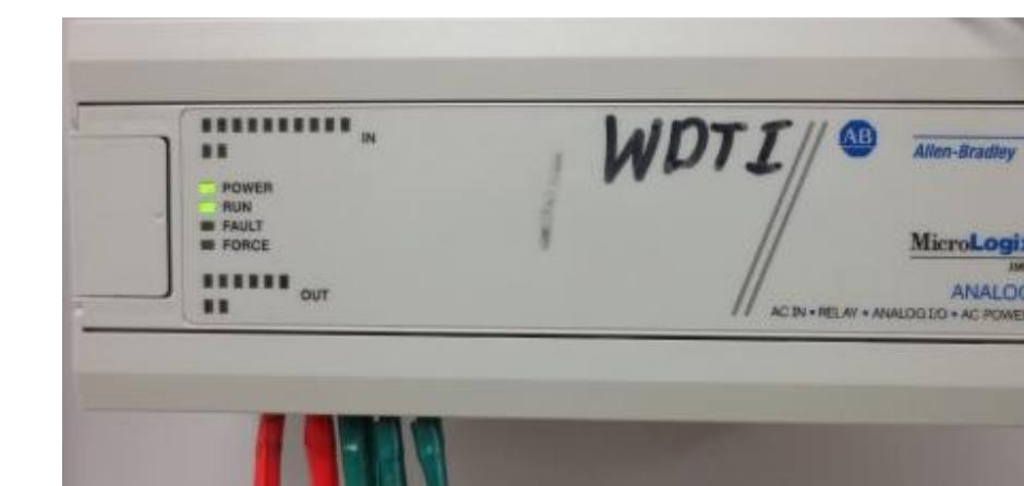
Image 4: Allen-Bradley MicroLogix 1000 PLC.
