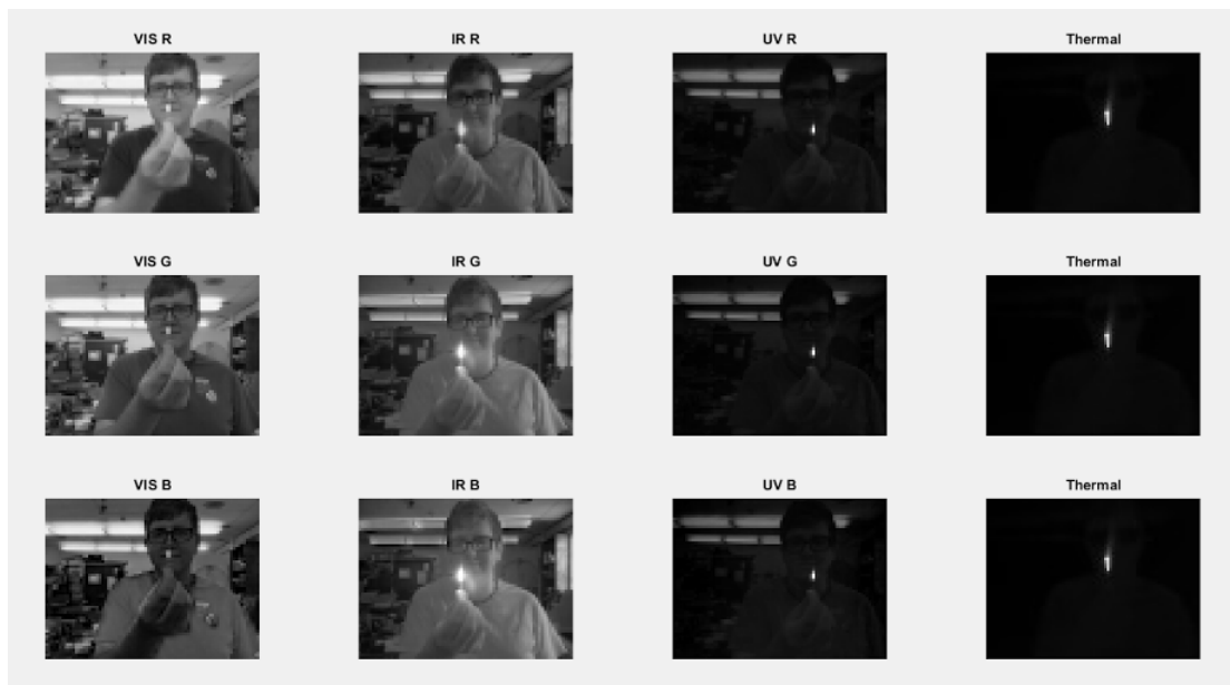
Figure 1: A test was conducted with an open flame (guaranteed to generate a response in UV, Thermal, Visual, IR, and NIR bands).
