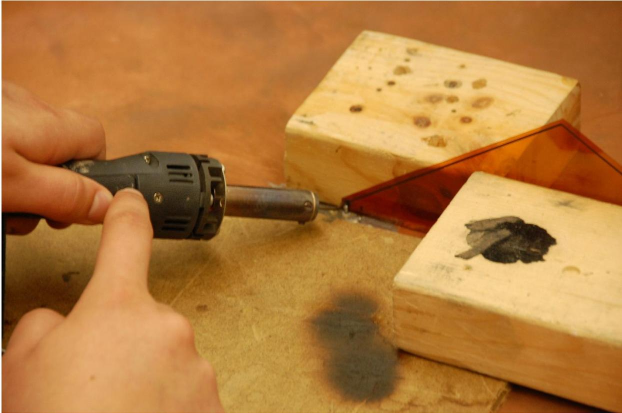
**Figure 4: A picture of the 35° ink-based (CI-2002) antenna curing to the ground plane.**
