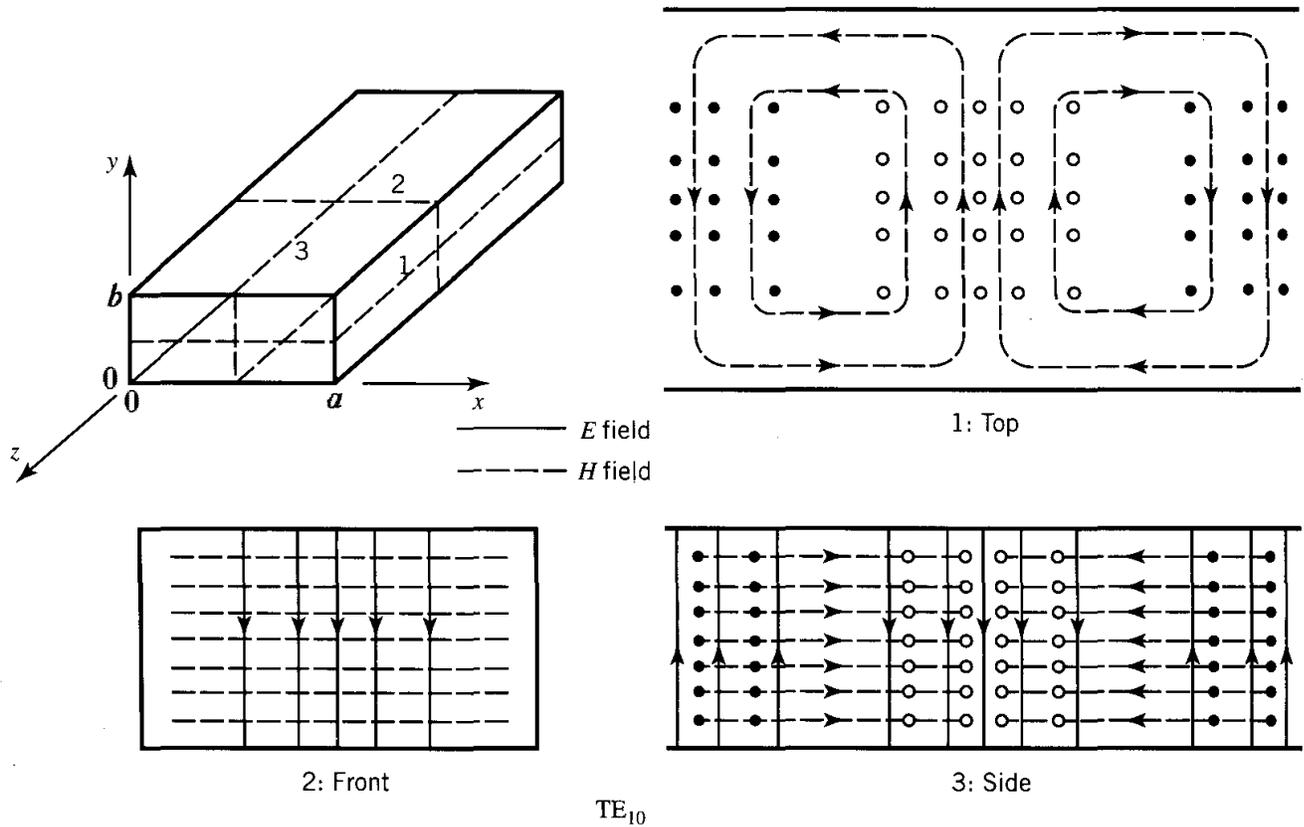
**Figure 8-7** Electric field patterns for  $TE_{10}$  mode in a rectangular waveguide. (Source: S. Ramo, J. R. Whinnery, and T. Van Duzer, *Fields and Waves in Communication Electronics*, 1984. Reprinted with permission of John Wiley & Sons, Inc.).
