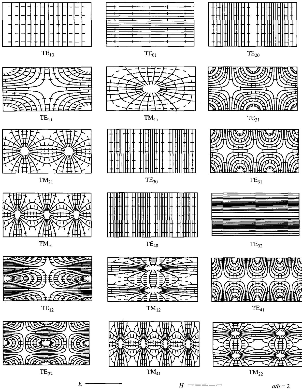
**Figure 8-6** Field patterns for the first 18  $TE^z$  and/or  $TM^z$  modes in a rectangular waveguide with  $a/b = 2$ . (Source: C. S. Lee, S. W. Lee, and S. L. Chuang, "Plot of modal field distribution in rectangular and circular waveguides," *IEEE Trans. Microwave Theory Tech.*, © 1985, IEEE.).
