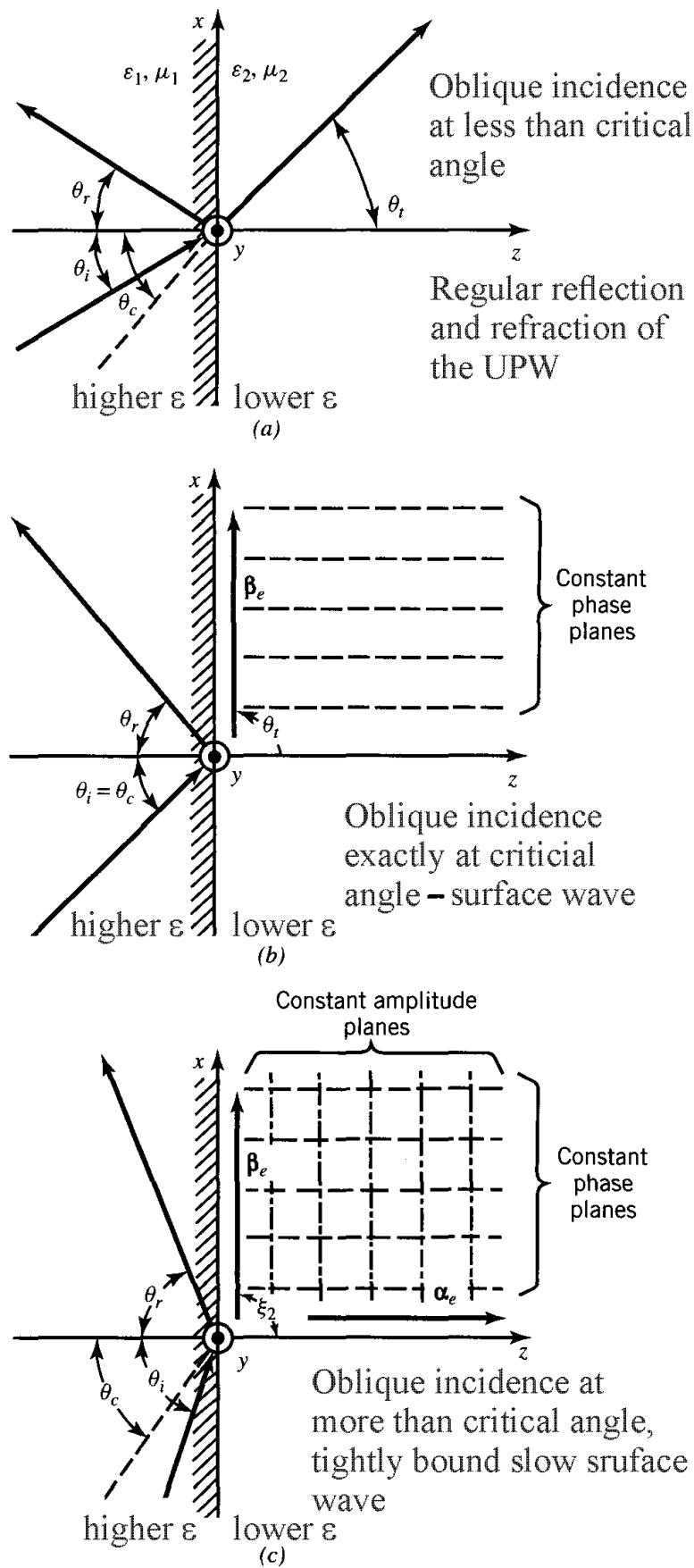
**Figure 5-7** Critical angle wave propagation along an interface.
