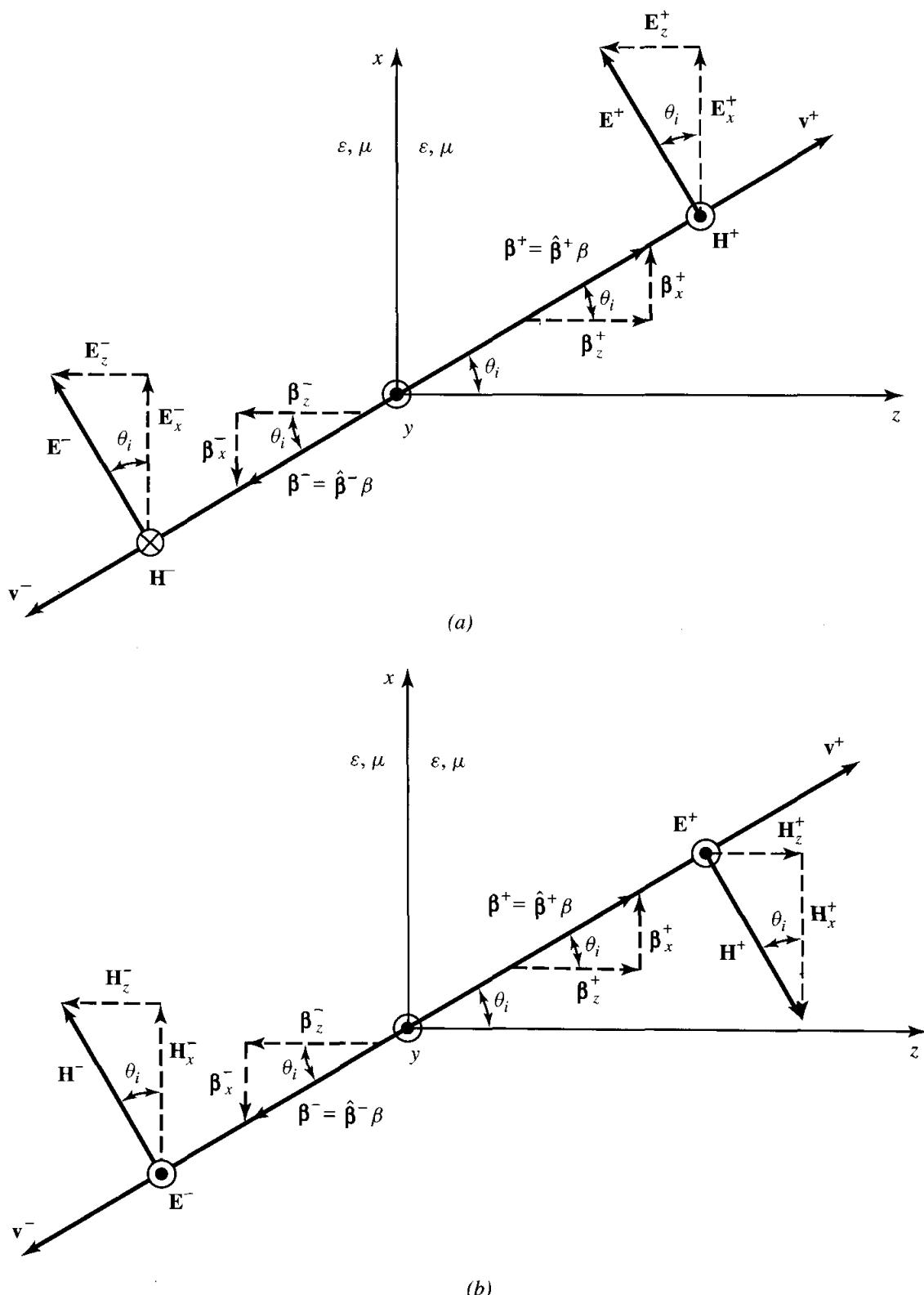
**Figure 4-4** Transverse electric and magnetic uniform plane waves in an unbounded medium at an oblique angle. (a) TE<sup>y</sup> mode. (b) TM<sup>y</sup> mode.
