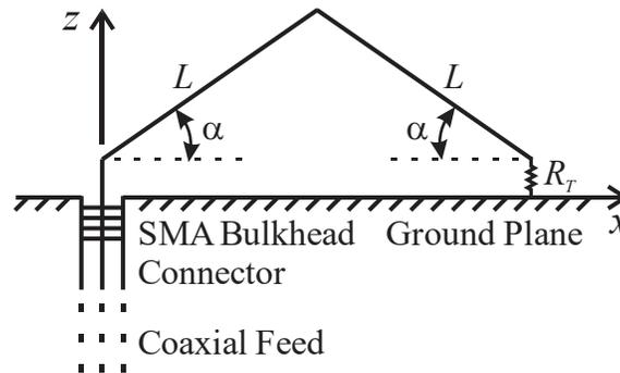
**Figure 1** Rhombic antenna geometry (not to scale)
