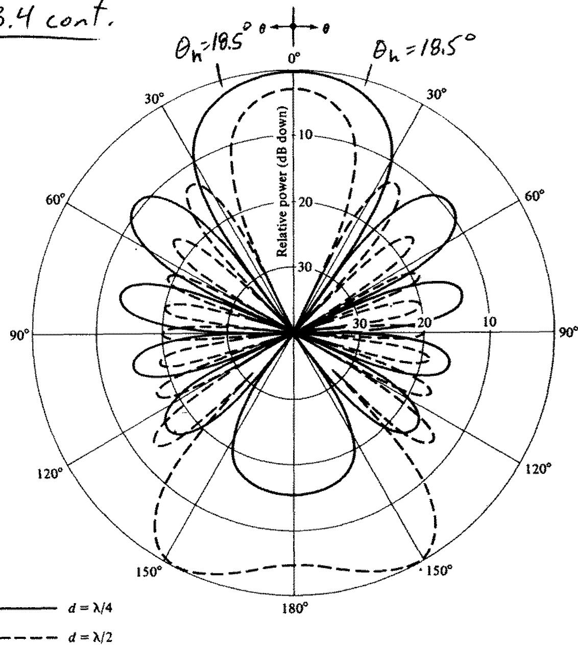
**Figure 6.12** Array factor patterns of a 10-element uniform amplitude Hansen-Woodyard end-fire array [ $N = 10$ ,  $\beta = -(kd + \pi/N)$ ] [Antenna Theory (Second Edition) by Balanis]
