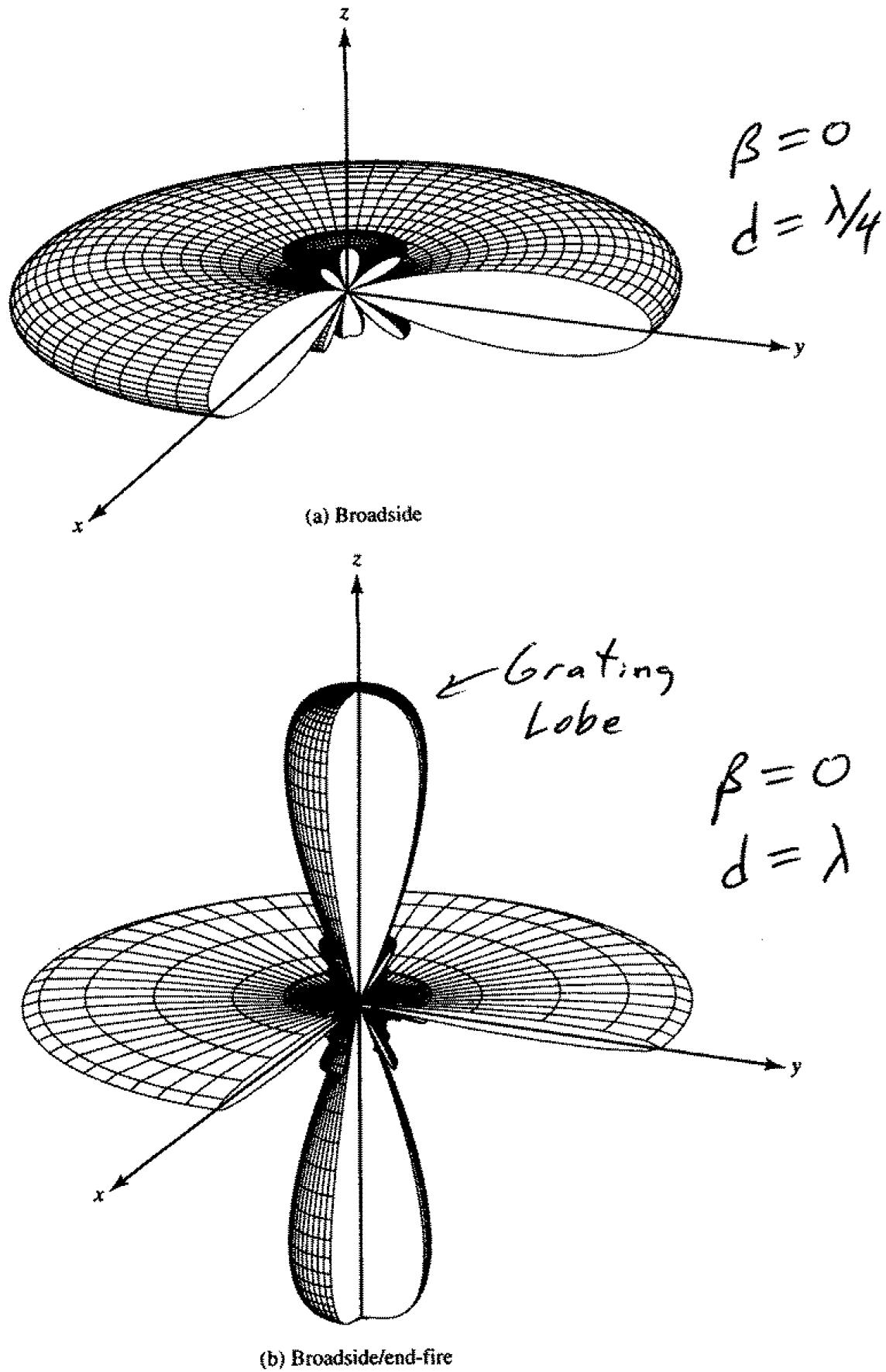
**Figure 6.6** Three-dimensional amplitude patterns for broadside, and broadside/end-fire arrays. [Antenna Theory (Second Edition) by Balanis]
