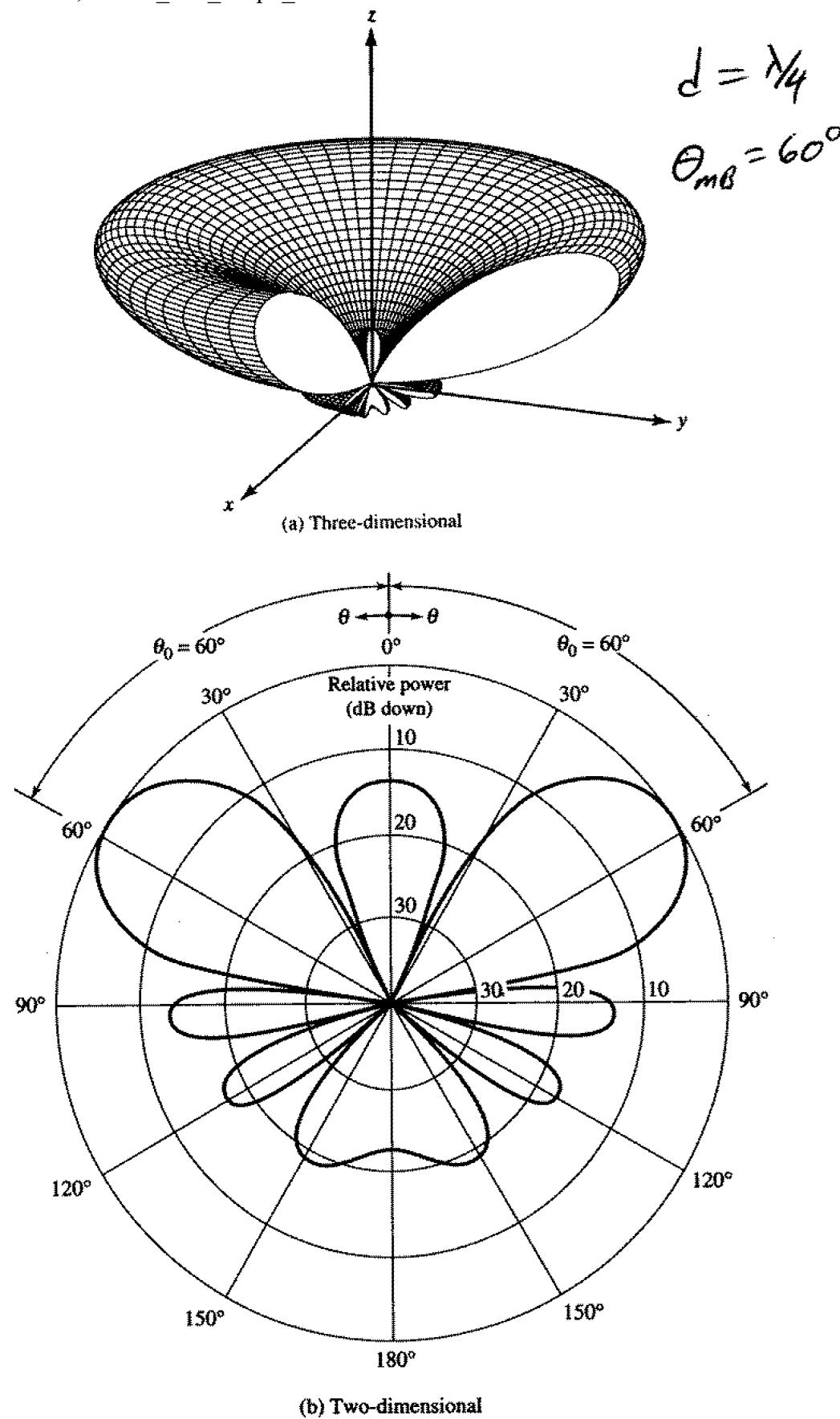
**Figure 6.10** Three- and two-dimensional array factor patterns of a 10-element uniform amplitude scanning array ( $N = 10$ ,  $\beta = -kd \cos \theta_0$ ,  $\theta_0 = 60^\circ$ ,  $d = \lambda/4$ .) [Antenna Theory (Second Edition) by Balanis]
