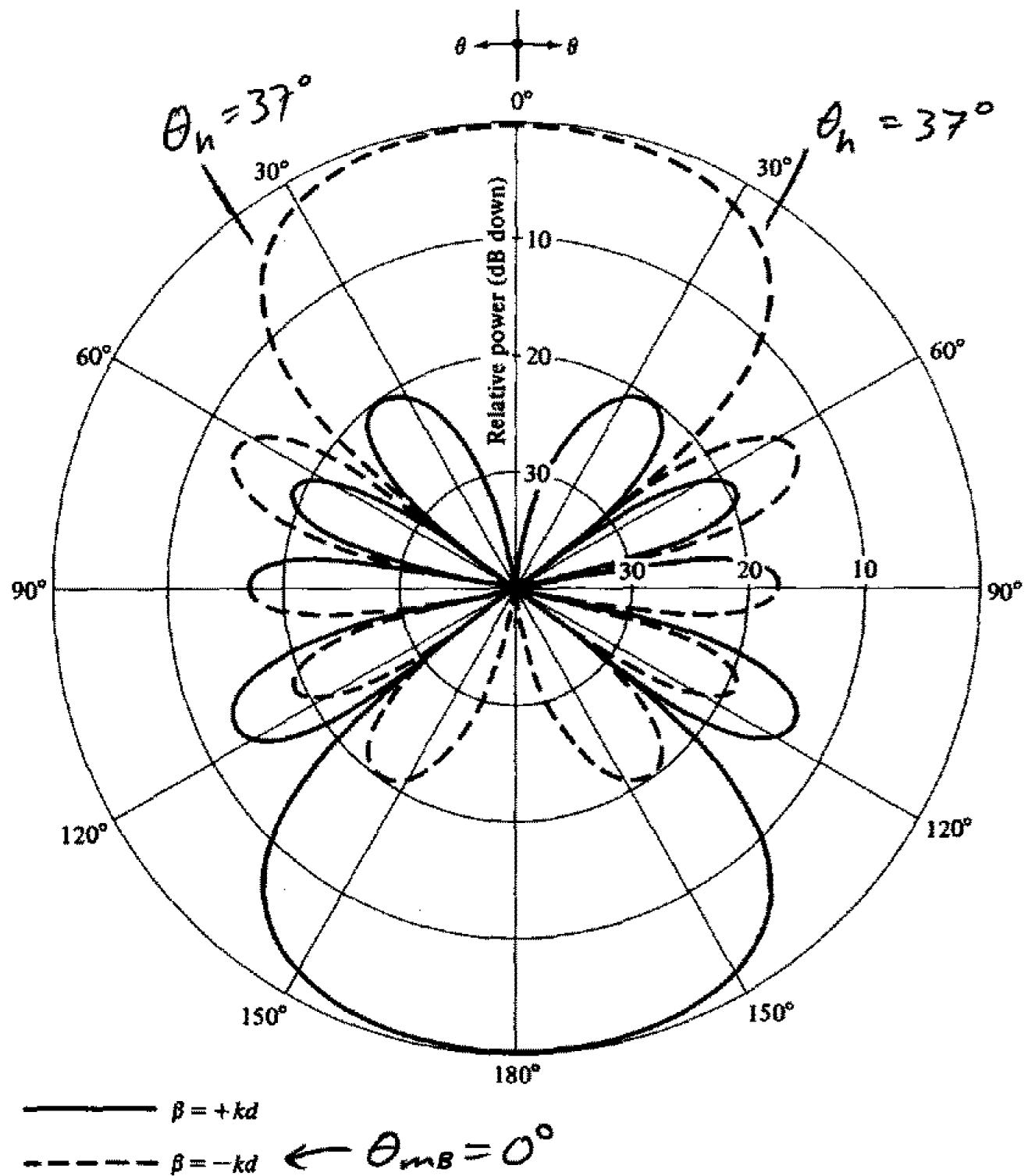
**Figure 6.9** Array factor patterns of a 10-element uniform amplitude end-fire array ( $N = 10, d = \lambda/4$ ). [Antenna Theory (Second Edition) by Balanis]
