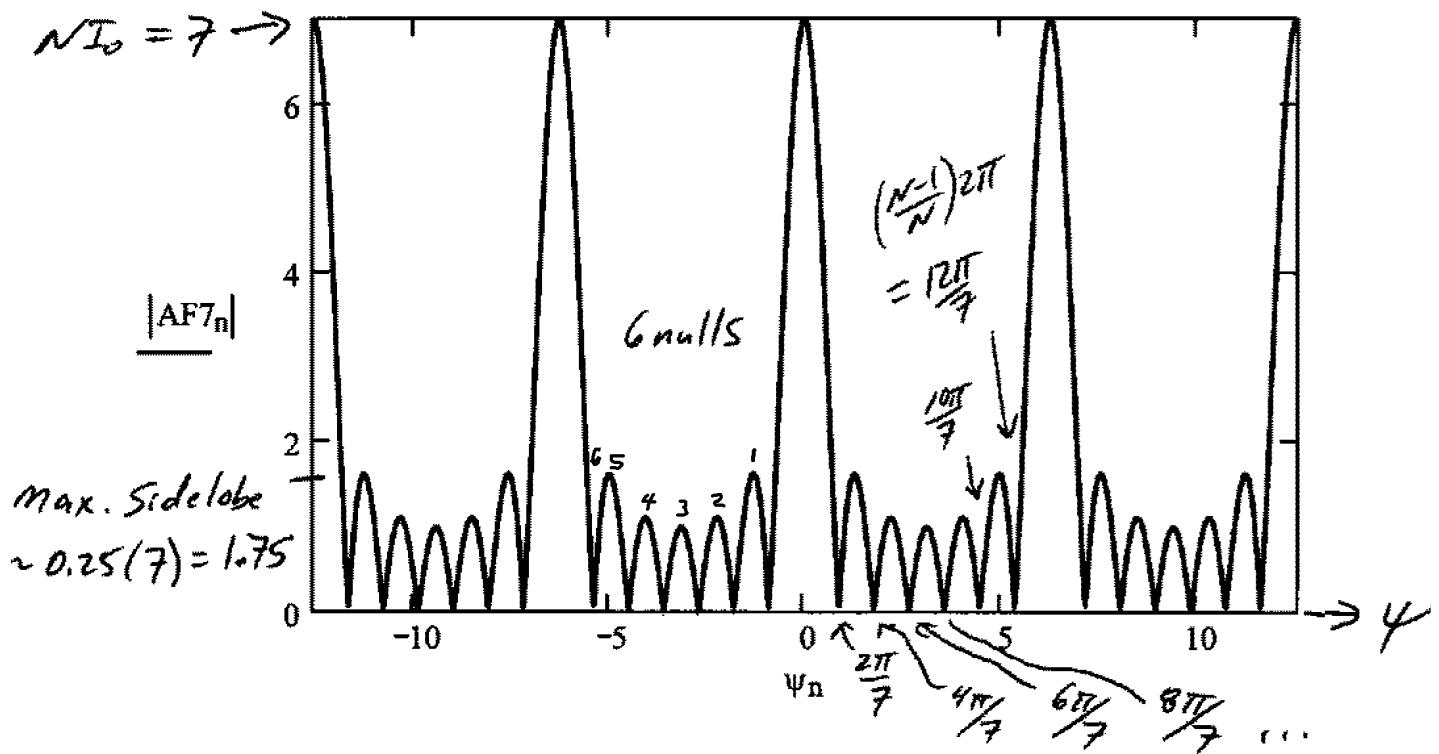
→ Main Beam narrower than  $N=4$  case
