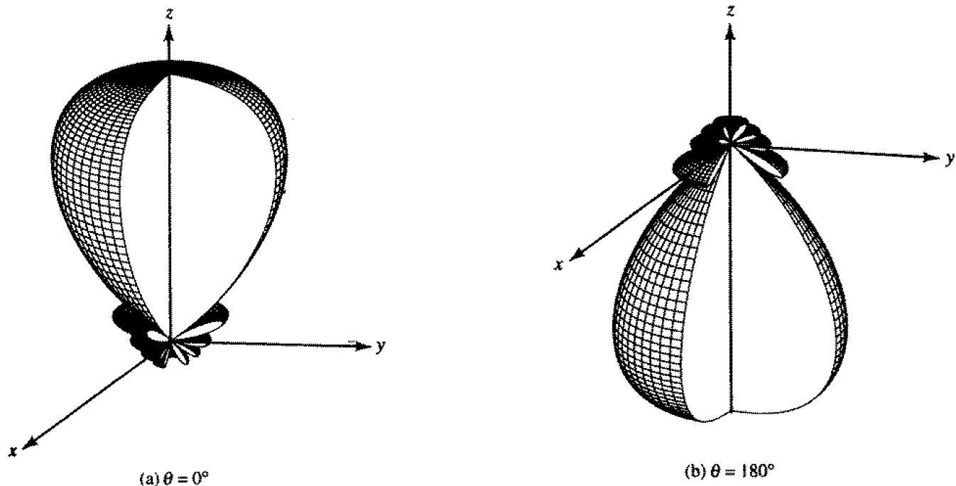
**Figure 6.8** Three-dimensional amplitude patterns for end-fire arrays toward  $\theta = 0^\circ$  and  $180^\circ$ . [Antenna Theory (Second Edition) by Balanis]
