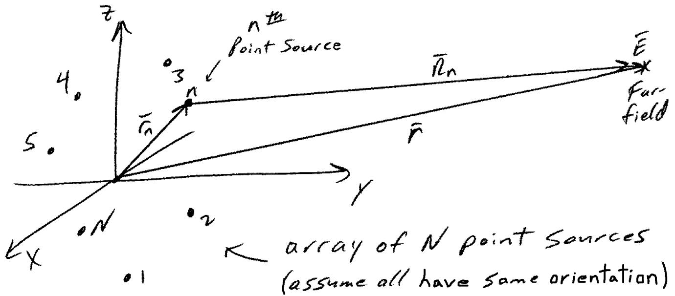
Assuming no interaction between the point sources, the far-field  $\bar{E}$  is simply the superposition of the far-fields for each point source
