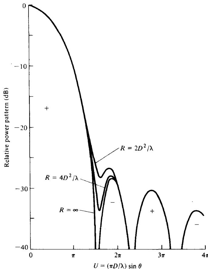
**Figure 2.9** Calculated radiation patterns of a paraboloid antenna for different distances from the antenna. (SOURCE: J. S. Hollis, T. J. Lyon, and L. Clayton, Jr. (eds.), *Microwave Antenna Measurements*, Scientific-Atlanta, Inc., July 1970).
