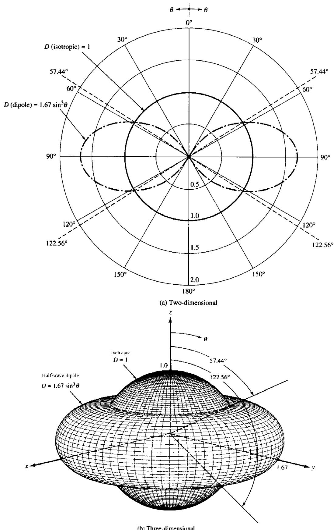
**Figure 2.13** Two- and three-dimensional directivity patterns of a  $\lambda/2$  dipole. (SOURCE: C. A. Balanis, "Antenna Theory: A Review." *Proc. IEEE*, Vol. 80, No. 1, January 1992. © 1992 IEEE.)
