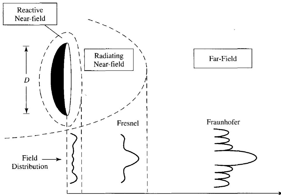
**Figure 2.8** Typical changes of antenna amplitude pattern shape from reactive near field toward the far field. (SOURCE: Y. Rahmat-Samii, L. I. Williams, and R. G. Yoccarino, "The UCLA Bi-polar Planar-Near-Field Antenna Measurement and Diagnostics Range," *IEEE Antennas & Propagation Magazine*, Vol. 37, No. 6, December 1995 © 1995 IEEE).
