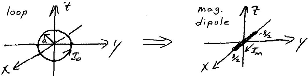
For the infinitesimal magnetic dipole, we evaluate the electric vector potential  $\bar{F}$
