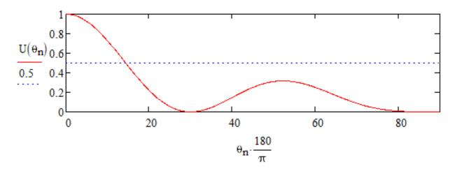
Using the graph as a starting point, find the angle  $\theta h$  where  $U(\theta h) = 0.5$  by trial and error to determine the HPBW.
