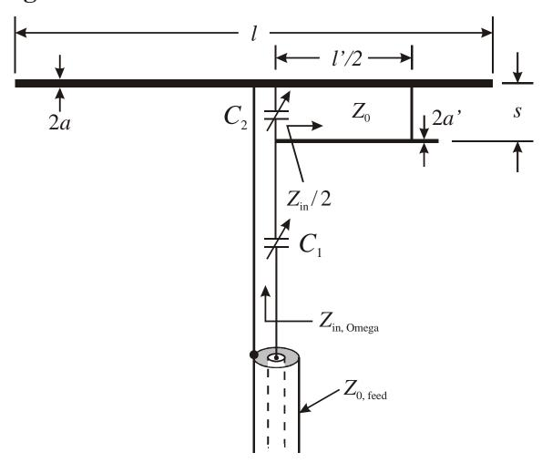
➤ The Omega-Match is a variation on the Gamma-Match that also allows the driven element of Yagi-Uda antennas to be fed by coaxial transmission lines (unbalanced).
