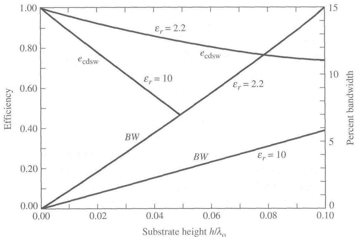
Figure 14.26 Efficiency and bandwidth versus substrate height at constant resonant frequency for rectangular microstrip patch for two different substrates ... (From Balanis, *Antenna Theory, Analysis and Design (Second Edition)*)
