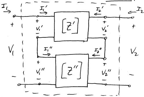
Since network [Z'] is in series with network [Z''],  $I_1' = I_1'' = I_1$  and  $I_2' = I_2'' = I_2$ . In addition, from KVL, we see that  $V_1 = V_1' + V_1''$  and  $V_2 = V_2' + V_2''$ .
