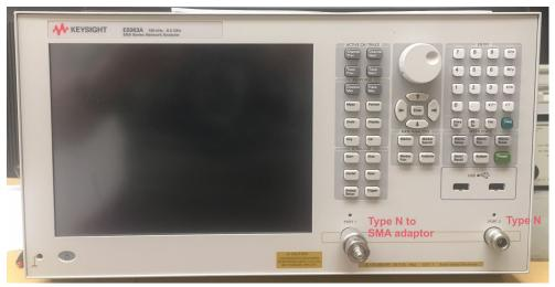
Note that the E5063A is a two port VNA with type N connectors. However, we will typically use a Type N to SMA adaptor to match our cables. For one port calibrations, we will use an Agilent 85033E 3.5 mm Calibration Kit. (below).
