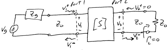
From  $[V^{-}] = [S][V^{\dagger}], we get$   $V_{1}^{-} = S_{11} V_{1}^{\dagger} + S_{12} V_{2}^{\dagger}$  $V_{2}^{-} = S_{21} V_{1}^{\dagger} + S_{22} V_{2}^{\dagger}$
