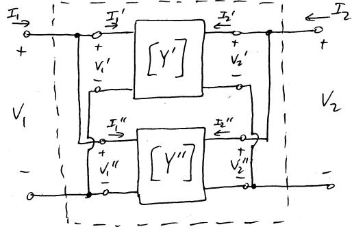
Since networks (Y') and (Y'') are connected in parallely  $V_1 = V_1'' = V_1''$  and  $V_2 = V_2'' = V_2''$ .
