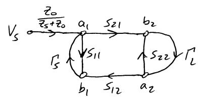
By definition,  $\Gamma_{in} \equiv \frac{b_1}{a_1}$ . So, we need to reduce the SFG to a point where there is a single branch to b, from  $a_1$ .
