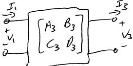
> We can replace two separate two-ports with a single equivalent two-port!
