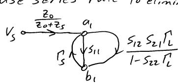
4.5 conti Step 5 Use parallel rule  $\frac{z_0}{z_0 + z_5} = a_1$   $V_5 = \frac{S_{11} + \frac{S_{12} S_{21} \Gamma_L}{1 - S_{22} \Gamma_L}}{1 - S_{22} \Gamma_L}$ We can now write  $b_1 = \left[ S_{11} + \frac{S_{12} S_{21} \Gamma_L}{1 - S_{22} \Gamma_L} \right] a_1$ .  $\Gamma_{1n} = \frac{b_1}{a_1} = S_{11} + \frac{S_{12} S_{21} \Gamma_L}{1 - S_{22} \Gamma_L}$
