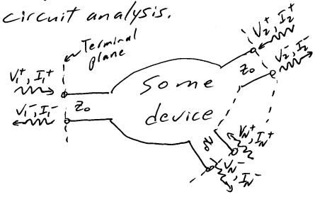
Here, Vnt are the complex amplitudes of the voltage waves incident at the ports. Whereas, Vn are the complex amplitudes of the voltage waves reflected, scattered, or emergins from the ports.
