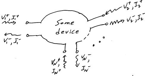
At each port of the device, we have both incident and reflected current & voltage waves. At the terminals (AKA: reference, phase, or terminal planes), the total current & voltage for the nth terminal is
