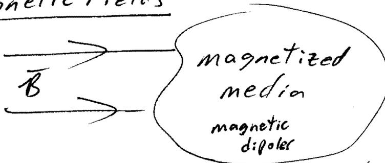
$$\bar{B} = \mu_0 (\bar{H} + \bar{M}) = \mu_0 (\bar{H} + \bar{P}_m) \quad \leftarrow \text{EE381/382} \quad \leftarrow \text{This text}$$
