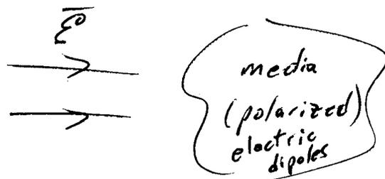
$$\vec{D} = \epsilon_0 \vec{E} + \vec{P} \quad \text{or} \quad \vec{D} = \epsilon_0 \vec{E} + \vec{P} \quad \text{Polarization vector (C/m}^2\text{)}$$
