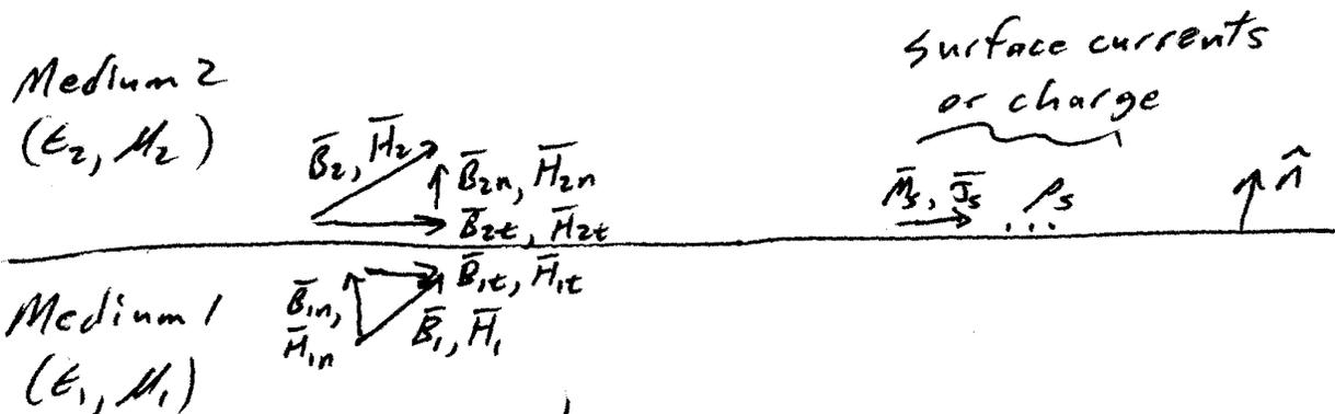
We can decompose fields into normal & tangential components
