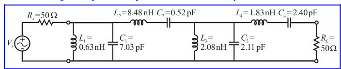
c) From circuits, use  $Z_R = R$ ,  $Z_L = j\omega L$ , and  $Z_C = -j/\omega C$ .
