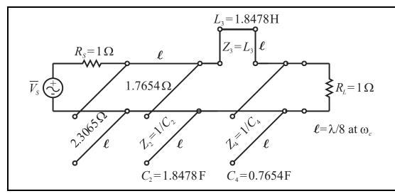
d) Add a unit element to the righthand side by load, sketch resulting circuit, apply Kuroda identity, & sketch resulting circuit.
