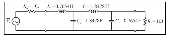
b) Using Richards' transformation (Fig. 8.34), we make the series inductors into series short circuit stubs & shunt capacitors into shunt open circuit stubs, both of length  $\ell = \lambda/8$  @  $\omega_c$ .
