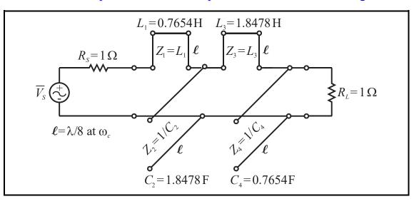
c) Add unit element to the lefthand side, sketch resulting circuit, apply Kuroda identity, & sketch resulting circuit.
