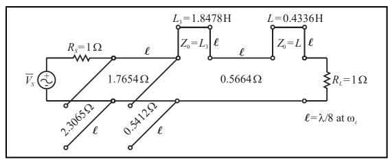
e) Add a unit element to the righthand side by load (again), sketch resulting circuit, apply Kuroda identity (b) to each of the two resulting short-circuit stub & unit element combinations, and sketch resulting circuit.
