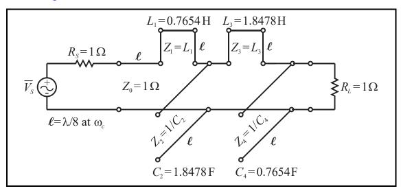
For LH unit element w/ series inductive SC stub combination, use Kuroda identity (a), let  $Z_1/n^2 = 0.7654 \Omega$ ,  $Z_2/n^2 = 1 \Omega$ , and  $n^2 = 1 + Z_2/Z_1 = 1 + 1/0.7654 = 2.3065$ . Therefore, we will get a TL section with impedance  $Z_1 = n^2(Z_1/n^2) = 2.3065(0.7654) = 1.7654 \Omega$  and a shunt capacitor of  $1/Z_2 = 1/[n^2 (Z_2/n^2] = 1/(2.3065*1) = 0.4336$  F. In turn, this shunt capacitor becomes a shunt OC stub of impedance  $Z_0 = 1/C = 1/0.4336 = 2.3065 \Omega$ .
