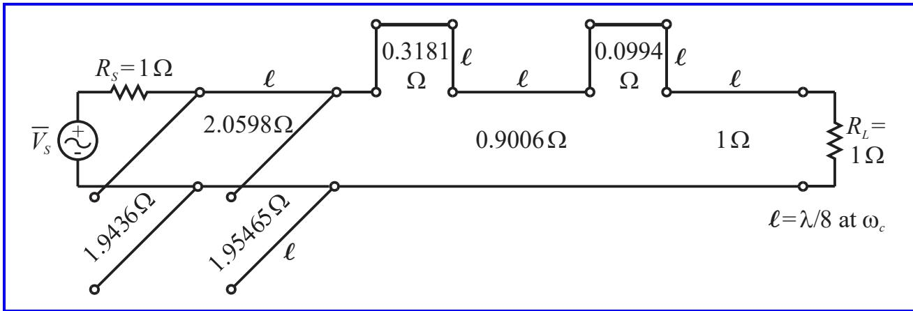
Apply Kuroda identity (b), shown below, to each of the two short-circuit series stub & unit element combinations to convert them to shunt stubs, and sketch resulting circuit. [Note: Normalized design should now only have shunt open-circuit stubs.]
