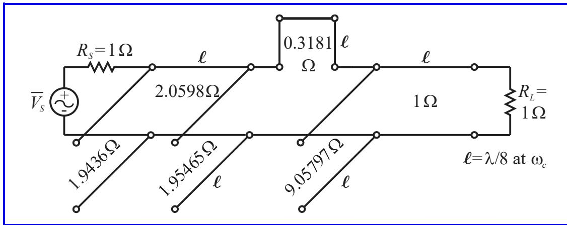
For RH unit element w/ shunt capacitive OC stub combination, use Kuroda identity (a), shown below, where  $Z_1 = 1 \Omega$ ,  $Z_2 = 1/0.1104 = 9.05797 \Omega$ , and  $n^2 = 1 + Z_2/Z_1 = 1 + 9.05797/1 = 10.05797$ . Here, the series SC stub has impedance  $Z_1/n^2 = 1/10.058 = 0.0994236 \Omega$  and the unit cell has impedance  $Z_2/n^2 = 9.05797/10.05797 = 0.900576 \Omega$ .
