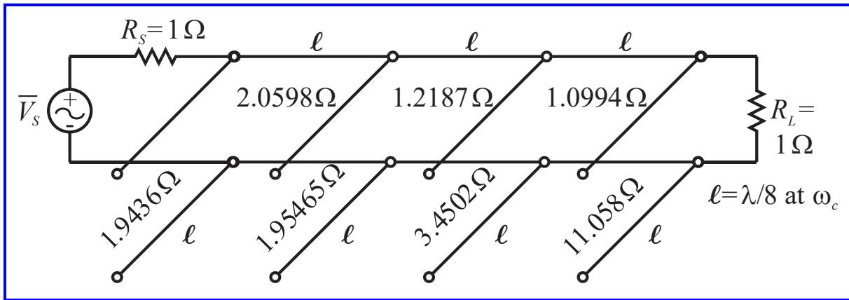
f) Scale all impedances to a  $50 \Omega$  system and draw a fully-labeled sketch of the final design [add  $50 \Omega$  sections (no specified length) at both ends for connectivity].
