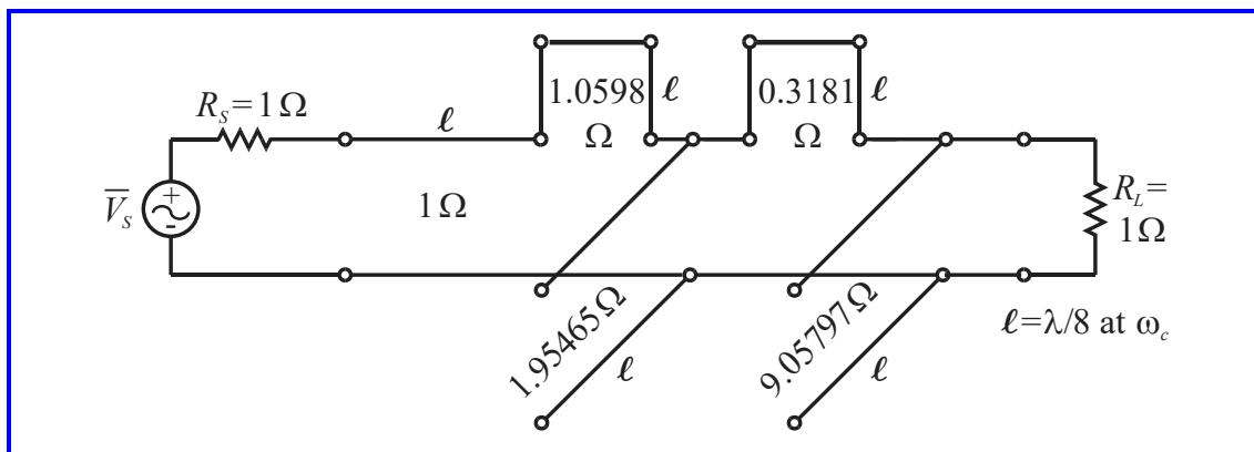
For LH unit element w/ series inductive SC stub combination, use mirrored Kuroda identity (b), shown below, where  $Z_2 = 1 \Omega$ ,  $Z_1 = 1.0598 \Omega$ , and  $n^2 = 1 + Z_2/Z_1 = 1 + 1/1.0598 = 1.94357$ . Here, the shunt OC stub has impedance  $n^2 Z_2 = 1.94357(1) = 1.94357 \Omega$  and the unit cell has impedance  $n^2 Z_1 = 1.94357(1.0598) = 2.0598 \Omega$ .
