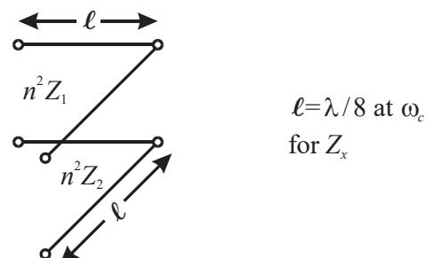
For the middle series inductive SC stub ( $Z_1 = 0.3181 \Omega$ ) with  $Z_2 = 0.900576 \Omega$  unit element combination,  $n^2 = 1 + Z_2/Z_1 = 1 + 0.900576/0.3181 = 3.83111$ . Therefore, we get a unit cell TL section with impedance  $n^2 Z_1 = 3.83111(0.3181) = \underline{\underline{1.21868 \Omega}}$  and a shunt OC stub of impedance  $n^2 Z_2 = 3.83111(0.900576) = \underline{\underline{3.4502 \Omega}}$ .
