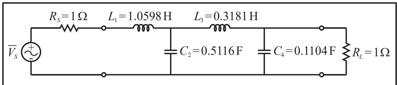
b) Using Richards' transformation (Fig. 8.34), the series inductors become series short circuit stubs & shunt capacitors become shunt open circuit stubs, all of length  $\ell = \lambda/8$  at  $\omega_c$ .
