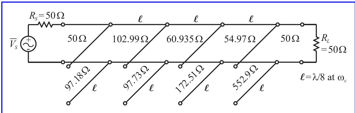
➤ The last  $553 \Omega$  OC stub is NOT practical, and the  $172.5 \Omega$  OC stub is borderline.
