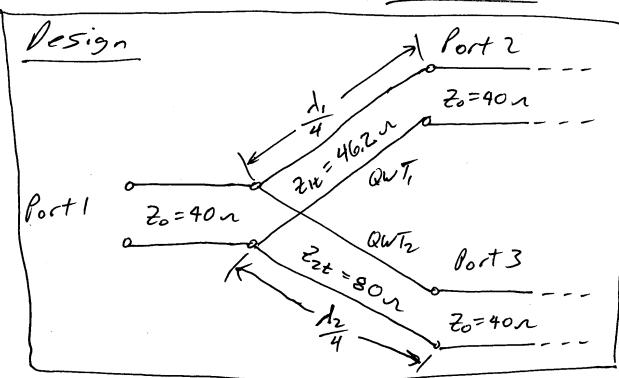
With ports 243 terminated in matched loads,  $S_{11} = I_{11} = \frac{z_{11} - z_{0}}{z_{11} + z_{0}} = \frac{40 - 40}{40 + 40} \Rightarrow |S_{11}| = 0$
