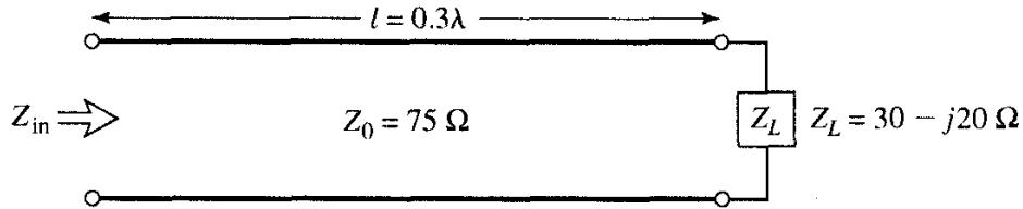
$$\text{Per (2.35), } \Gamma = \Gamma_L = \frac{Z_L - Z_0}{Z_L + Z_0} = \frac{(30 - j20) - 75}{(30 - j20) + 75} \Rightarrow \underline{\Gamma_L = 0.46071 \angle -145.2532^\circ}$$
