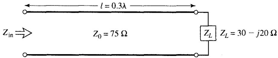
$$\text{Per (2.35), } \Gamma = \Gamma_L = \frac{Z_L - Z_0}{Z_L + Z_0} = \frac{(30 - j20) - 75}{(30 - j20) + 75} \Rightarrow \underline{\Gamma_L = 0.46071 \angle -145.2532^\circ}$$
