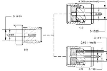
Figure 1: The single SMA female configuration (a) can mate with both the "conventional" male (b), and the "thru" male (c).
