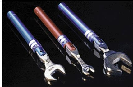
If you over-torque a connection, it is possible you will damage the connector on the vector network analyzer, the cable or your microwave circuit. There may be different types of torque wrenches lying about the lab. Be certain that you are using the **BLACK** colored torque wrench.
