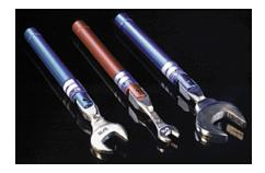
If you over-torque a connection, it is possible you will damage the connector on the vector network analyzer, the cable or your microwave circuit. There may be different types of torque wrenches lying about the lab. Be certain that you are using the BLACK colored torque wrench.
