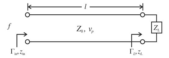
For the lossless transmission line circuit shown:  $f = 500 \,\text{MHz}$ ,  $v_p = 2 \times 10^8 \,\text{m/s}$ ,  $l = 1.242 \,\text{m}$ ,  $Z_0 = 75 \,\Omega$ , and  $\Gamma_{\text{in}} = 0.8 \angle -117.5^{\circ}$ .
