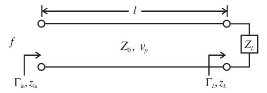
For the lossless transmission line circuit shown:  $f = 100 \,\text{MHz}$ ,  $v_p = 3 \times 10^8 \,\text{m/s}$ ,  $l = 3.3 \,\text{m}$ ,  $Z_0 = 50 \,\Omega$ , and  $Z_L = 75 + j \,50 \,\Omega$ .
