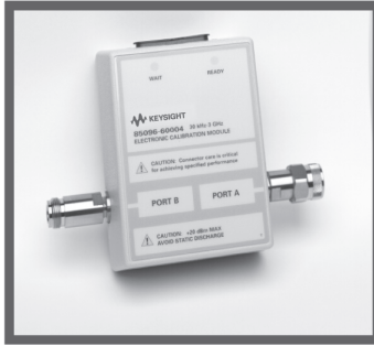
Microwave modules use a transmission line shunted by PIN-diode switches in various combinations
