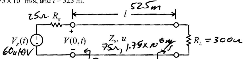
$$\Gamma_L = \frac{Z_L - Z_0}{Z_L + Z_0} = \frac{300 - 75}{300 + 75} = 0.6; \quad \Gamma_g = \frac{Z_0 - Z_0}{Z_0 + Z_0} = \frac{75 - 75}{75 + 75} = -0.5$$
