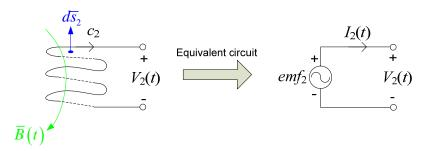
Notice here that the direction of  $d\overline{s}_2$  (dictated by the given direction for  $I_2$  and hence  $c_2$ ) is <u>opposite</u> that of  $\overline{B}$ . Consequently, from the equivalent circuit and using (4) again we determine that
