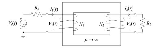
This transformer "transforms" the load resistance to the primary according to (12). An equivalent circuit at the primary terminal can be constructed using this effective primary resistance:
