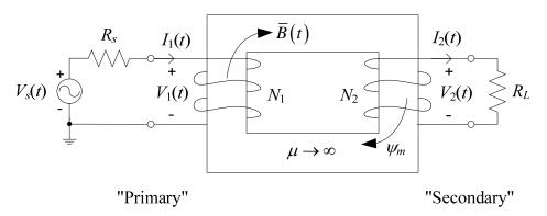
Notice that there is <u>no continuous path</u> for conduction current from the voltage source  $V_s$  to the load resistor  $R_L$ . These two ports instead are electrically "coupled" to each other indirectly by the principal of induction from Faraday's law.
