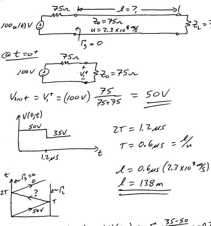
$$35V = 50V + \Gamma_{L}(50V) + O(\Gamma_{L})(50V) \Rightarrow \Gamma_{L} = \frac{35-50}{50} = -0.3$$
