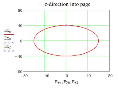
From plot, the **sense** of the polarization ellipse is **<u>RH</u>/righthand</u> or <u><b>CW**/clockwise</u>. From plot, the axial ratio  $AR = 2*60/2*40 = 120/80 \Rightarrow \underline{AR} = 1.5$ . From plot, the tilt angle  $\tau$  with respect to the vertical/ $E_x$  axis is  $\underline{\tau} = 90^\circ$ .
