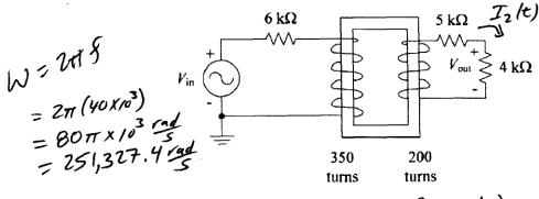
=> Ignore OC component of Vn(t) as it will NOT couple to the secondary side of the transformer
