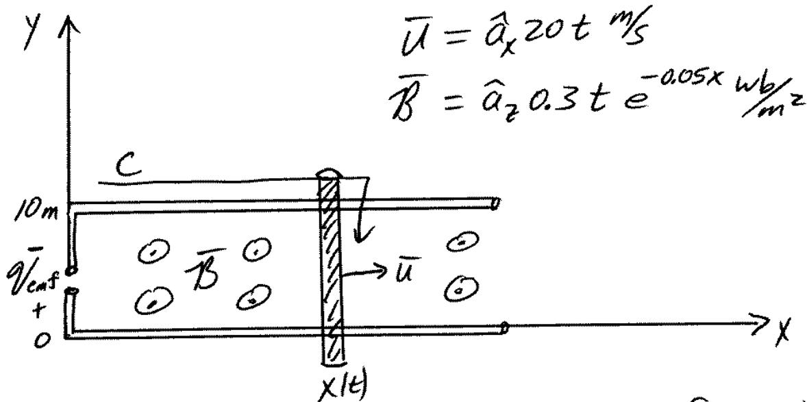
$$\underline{\text{Method 1}} \quad V_{\text{emf}} = \text{emf} = - \int \frac{d\bar{B}}{dt} \cdot d\bar{s} + \oint_c (\bar{u} \times \bar{B}) \cdot d\bar{l}$$
