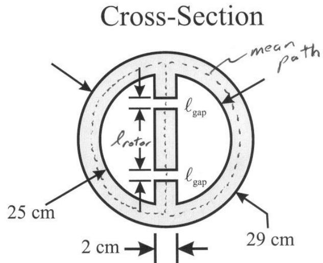
Given:  $\mu = 5000\mu_0$  for rotor & stator
