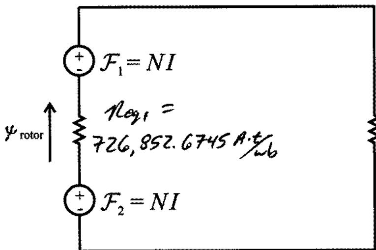
$$R_{eq2} = \frac{R_{stator}}{2} // \frac{R_{stator}}{2}$$
