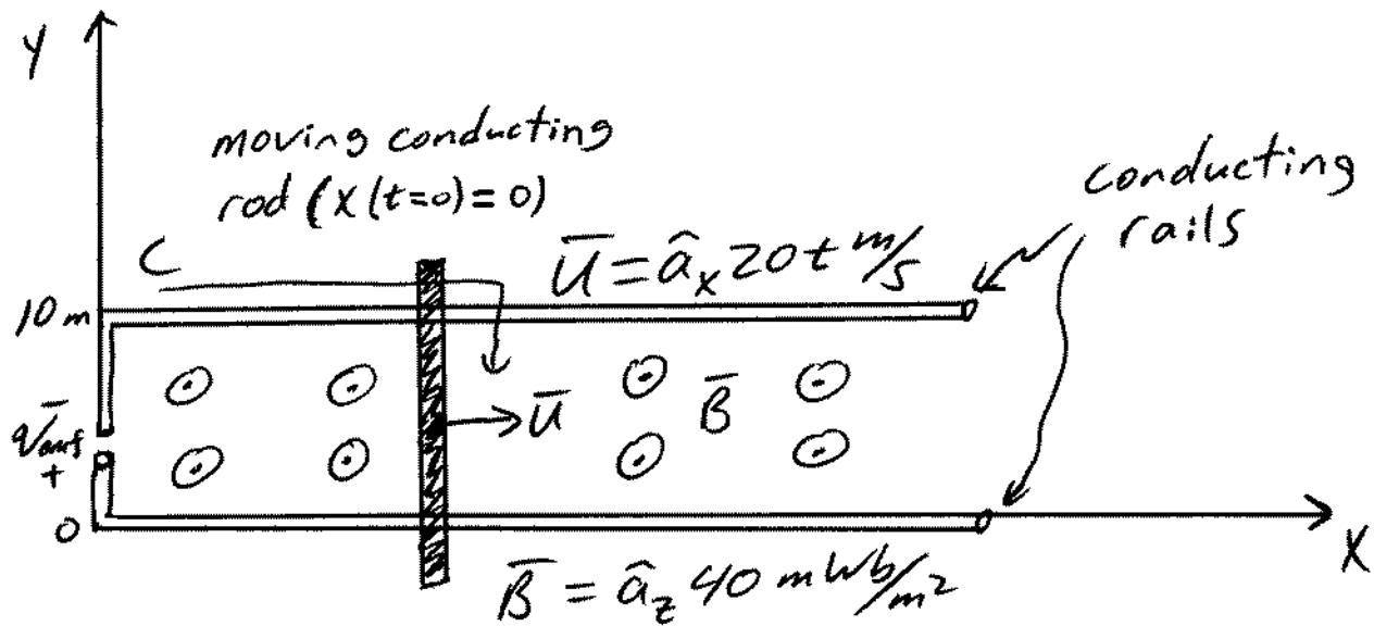
→ From Lenz's Law, we expect the emf to work CW around the contour to oppose the increase in  $\Phi_m$  as the rod moves to the right.
