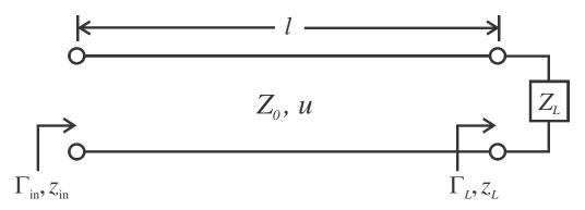
For the lossless transmission line circuit above, the frequency, length, and phase velocity will be left unspecified while  $Z_0 = 75 \Omega$  and  $Z_L = 56.25 - j75 \Omega$ .
