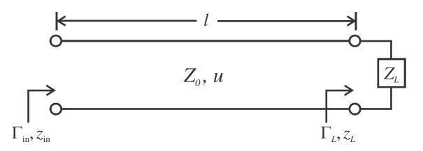
For the lossless transmission line circuit shown: f = 500 MHz,  $u = 2 \times 10^8 \text{ m/s}$ , l = 1.242 m,  $Z_0 = 75 \Omega$ , and  $\Gamma_{\text{in}} = 0.8 \angle -117.5^\circ$ .
