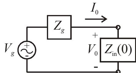
$$V_0 = V_g \left( \frac{Z_{\text{in}}(0)}{Z_g + Z_{\text{in}}(0)} \right) \text{ and } I_0 = \frac{V_g}{Z_g + Z_{\text{in}}(0)}.$$
