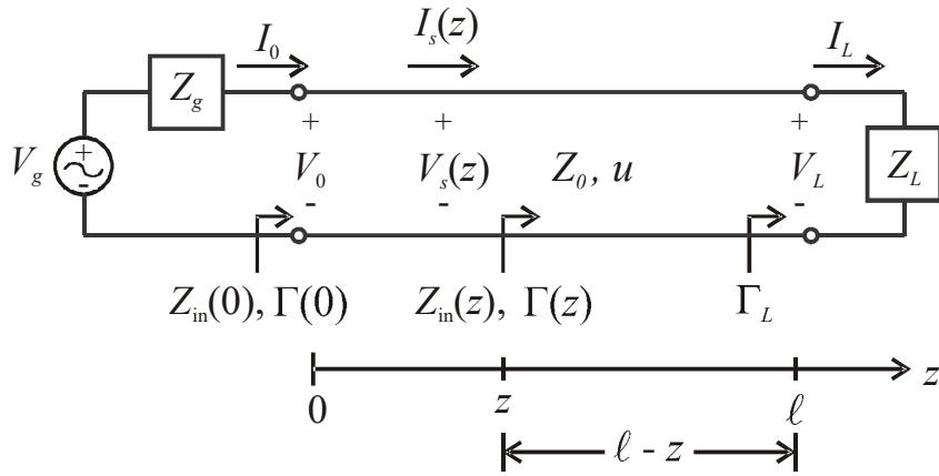
$$u = f\lambda = \frac{\omega}{\beta} = \frac{1}{\sqrt{LC}} \text{ (m/s)}, \quad \beta = \frac{\omega}{u} = \omega\sqrt{LC} = \frac{2\pi}{\lambda} \text{ (rad/m)}, \quad \lambda = \frac{u}{f} = \frac{2\pi}{\beta} \text{ (m)}$$
