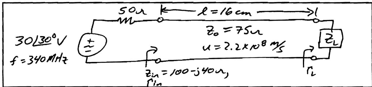
$$\beta = \frac{\omega}{u} = \frac{2\pi(340 \times 10^6)}{2.2 \times 10^8} = \underline{9.7104 \text{ rad/m}}$$
