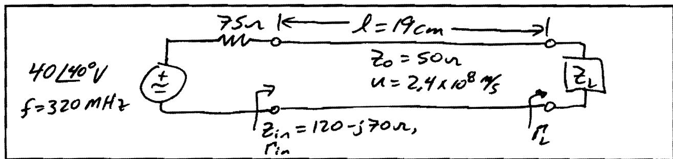
$$\beta = \frac{\omega}{u} = \frac{2\pi(320 \times 10^6)}{2.4 \times 10^8} = \underline{8.37750 \text{ rad/m}}$$
