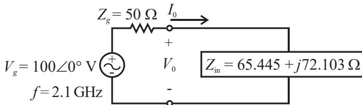
$$I_0 = \frac{V_g}{Z_g + Z_{\text{in}}} = \frac{100\angle 0^\circ}{50 + (65.445 + j72.103)} \Rightarrow I_0 = 0.73469\angle -31.987^\circ \text{ A}$$
