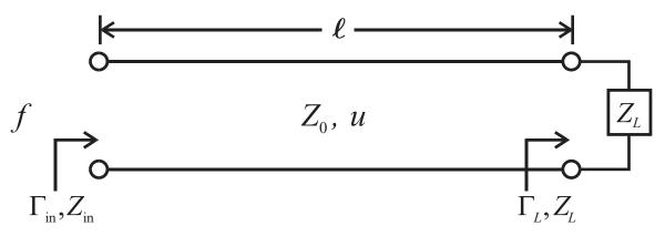
For the lossless transmission line circuit above, the frequency, length, and phase velocity will be left unspecified while  $Z_0 = 75 \Omega$  and  $Z_L = 56.25 - j75 \Omega$ .
