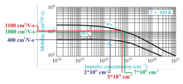
ho <u>n-type sample</u>: With  $N_i \approx N_d = 5 \times 10^{16} \, \text{\#/cm}^3$   $\Rightarrow \underline{\mu_n \approx 1100 \, \text{cm}^2/\text{V-s}}$
