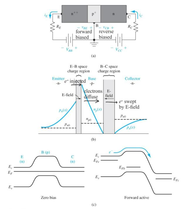
**Figure 12.4** I (a) Biasing of an npn bipolar transistor in the forward-active mode, (b) minority carrier distribution in an npn bipolar transistor operating in the forward-active mode, and (c) energy-band diagram of the npn bipolar transistor under zero bias and under a forward-active mode bias.
