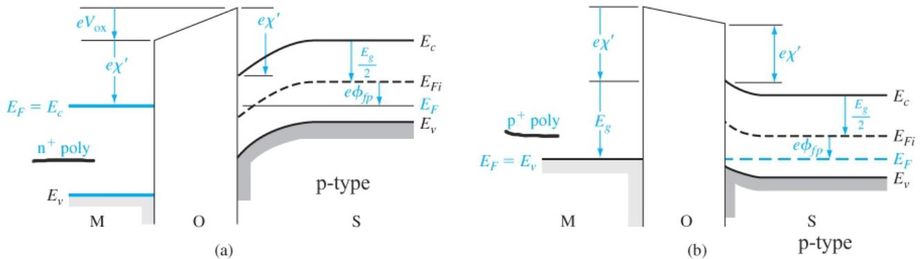
**Figure 10.14** | Energy-band diagram through the MOS structure with a p-type substrate at zero gate bias for (a) an n<sup>+</sup> polysilicon gate and (b) a p<sup>+</sup> polysilicon gate.
