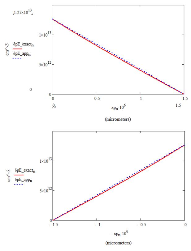
Note that the exact (12.21a) and approximate (12.21b) expressions yield very close results even though the emitter length is a significant fraction of the diffusion length, i.e.,  $x_E/L_E = 0.5576$ .
