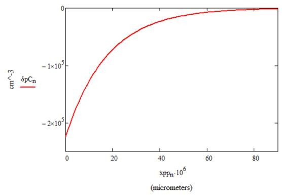
At  $x_C$ ,  $\delta p_C(90 \ \mu m) = -1.358 \ cm^{-3} \approx 0$ , i.e., 0.6% of  $\delta p_C(0)$ . So, the long collector approximation is close for  $x_C/L_C = 90/17.61 = 5.11$ .
