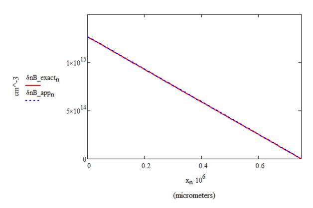
To the eye, the traces for the exact (12.15a) and approximate (12.15b) expressions for the excess minority carrier (electron) concentrations match exactly.
